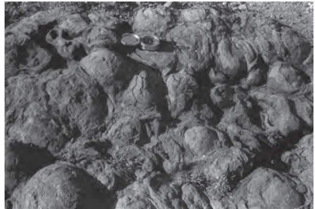
Fig.5.3 : Exfoliation (Flaking) and granular disintegration
