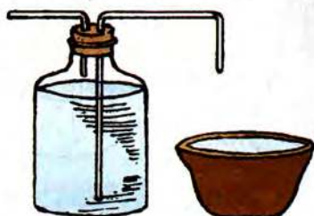
Fig. 14.11 An apparatus to measure the volume of air breathed out.
