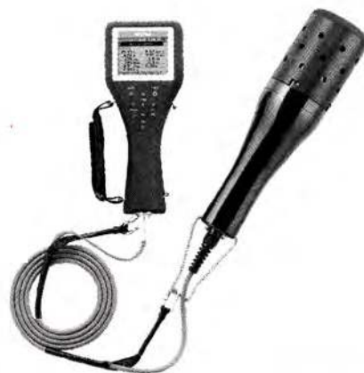
Fig. 9.6 Instrument for measuring dissolved oxygen
