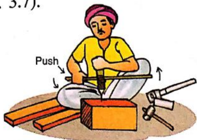
Fig. 3.7 Turning of a drill machine
