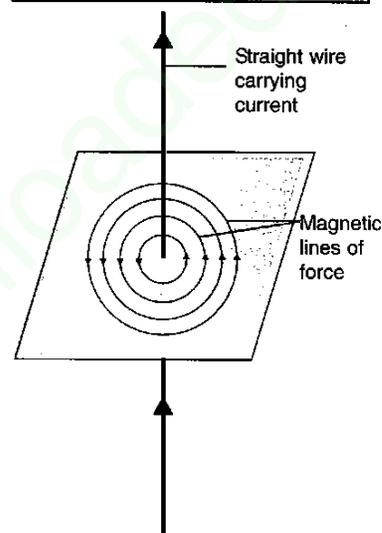
**Fig. 7.5** Magnetic field due to a straight wire carrying current
