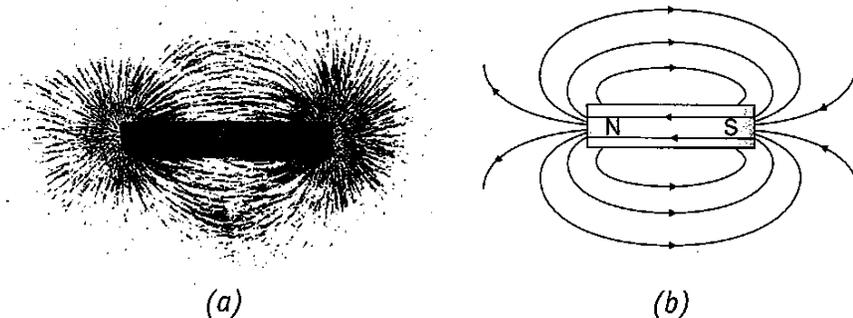
**Fig. 7.3** (a) Iron filings around a bar magnet; and (b) Magnetic lines of force around a bar magnet
