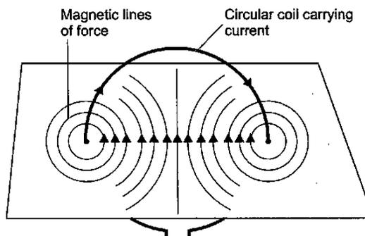
**Fig. 7.7** Magnetic field due to a circular coil carrying current
