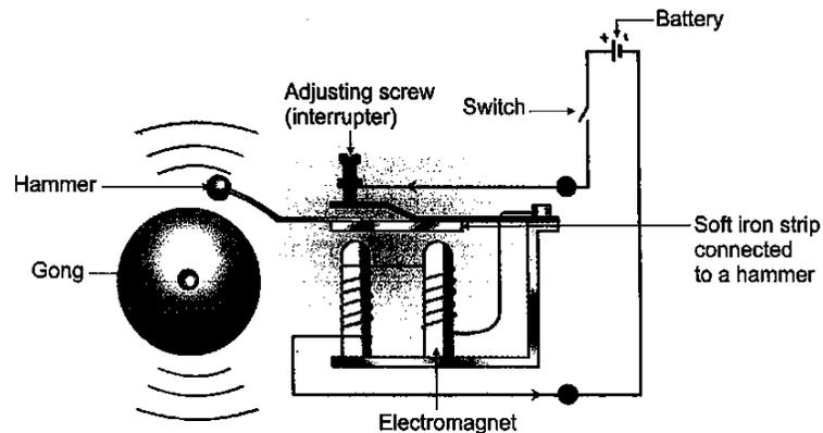
**Fig. 7.10** Working of an electric bell
