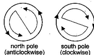
Fig. 7.9 Determining the poles of a solenoid
