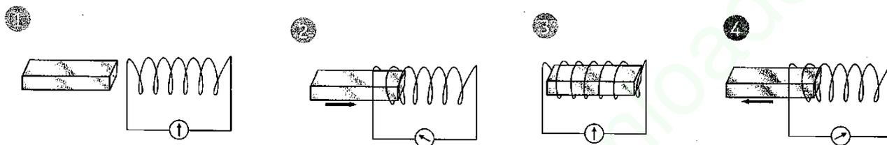
1. If a bar magnet is kept close to a wire and no movement of the magnet or the wire is made, the current does not flow in the wire and the galvanometer shows no deflection.
