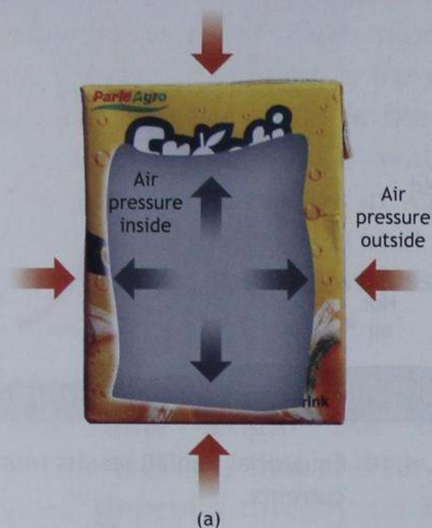
Fig. 4.11 (a) An empty carton is filled with air, so the pressure inside is balanced by the pressure outside. (b) When air is sucked out, the carton caves in because of the higher pressure outside.
