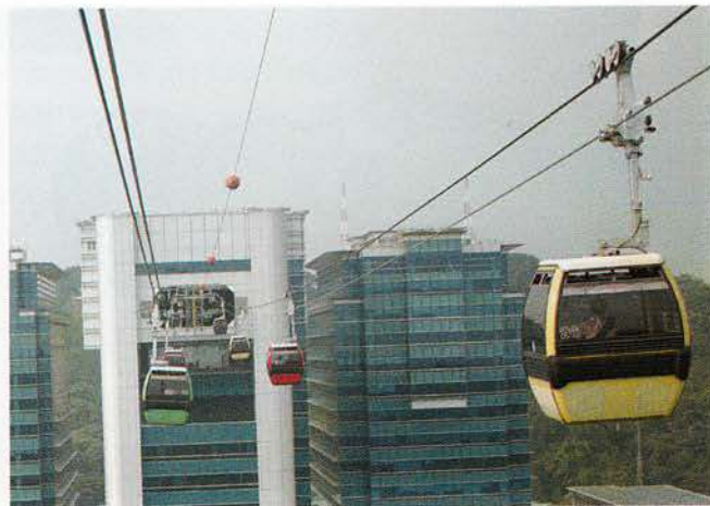
Fig. 6.2 Metals have high tensile strength. Steel cables carry heavy loads such as that of cable cars.
