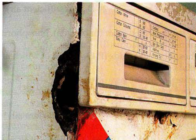
Fig. 6.7 Corrosion in the body of a washing machine
