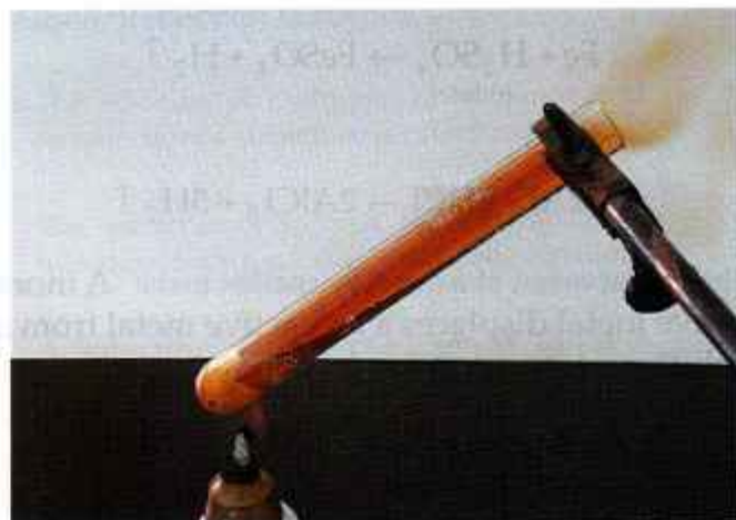
Fig. 5.16 On being heated, lead nitrate gives brown fumes of nitrogen dioxide.
