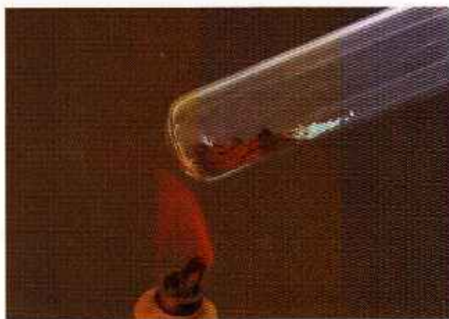
Fig. 5.11 On being heated, copper(II) carbonate (green) gives copper(II) oxide (black).
