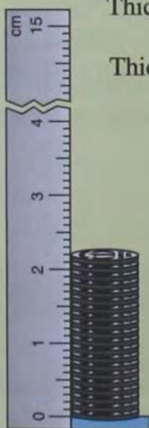
Fig. 1.8 Measuring the thickness of a stack of coins
