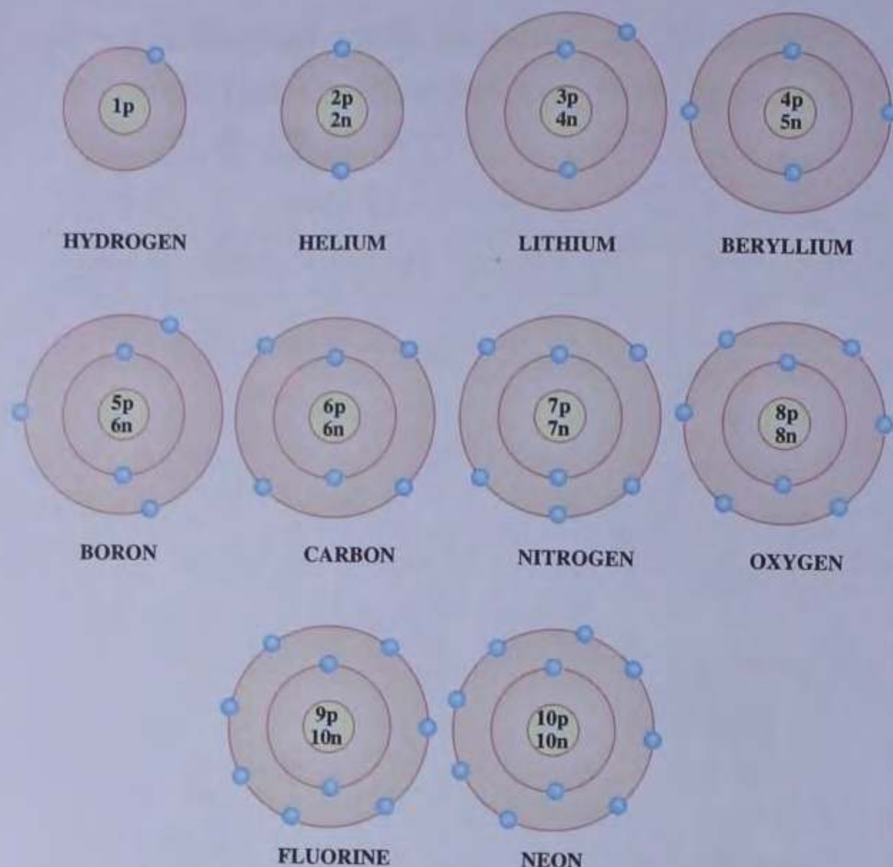
Fig. 2.4 Atomic diagrams of elements with atomic number (1-10) to show arrangement of electrons in different shells.
