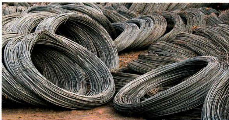
Fig. 6.2 Metals are ductile and malleable—they can be drawn into wires or pressed to form sheets or foils.
