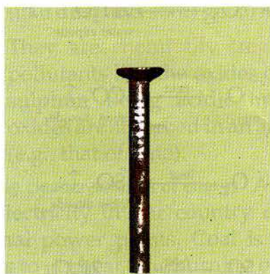
Fig. 4.2 Rusting of iron
