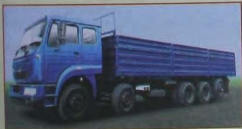
Heavy trucks have more tyres to reduce pressure on the road
