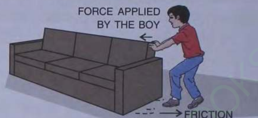
Fig. 2.11 Friction opposes the motion
