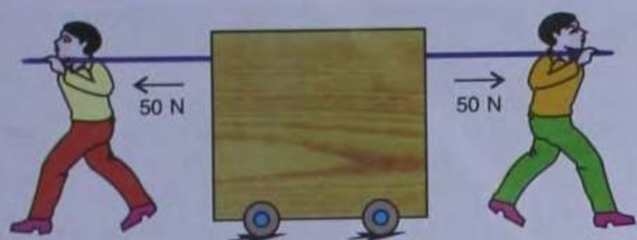
Fig. 2.22 Two equal and opposite forces – the net force is zero
