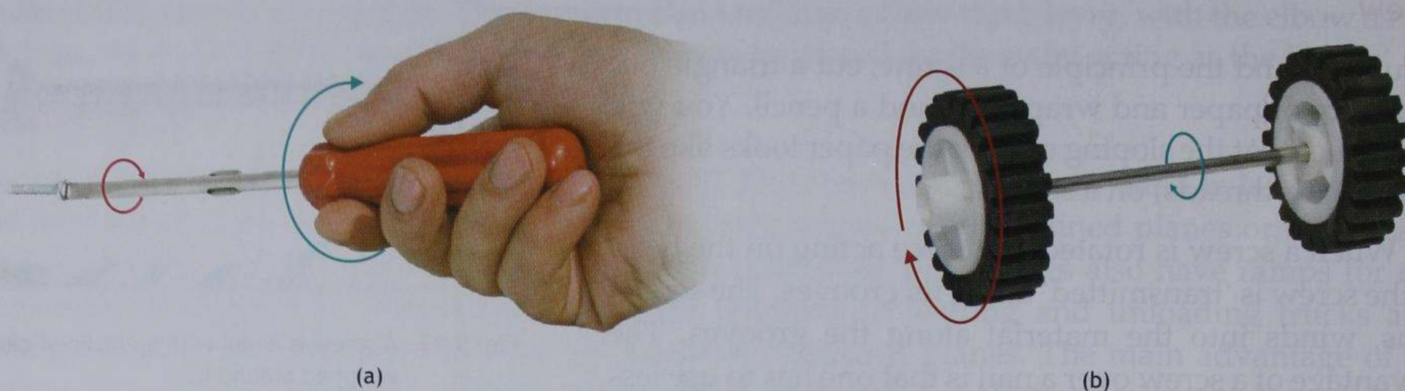
Fig. 5.15 The wheel-and-axle arrangement can be used (a) to magnify force or (b) to magnify movement.
