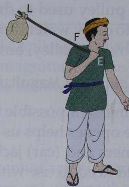
Fig. 5.6 The basic parts of a lever
