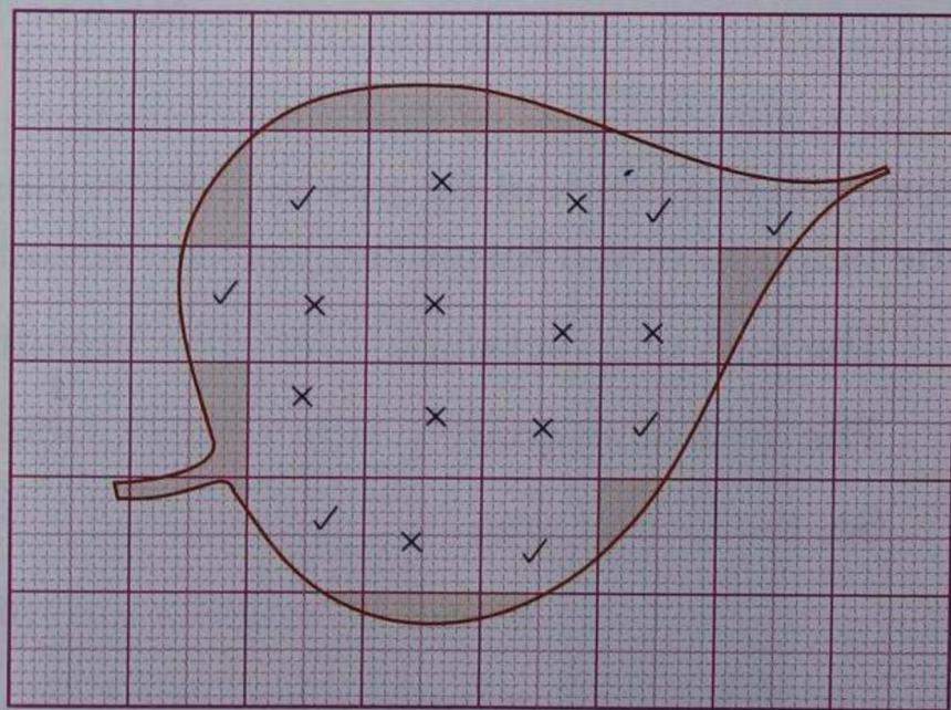
Fig. 2.10 Measuring the area of an irregular shape
