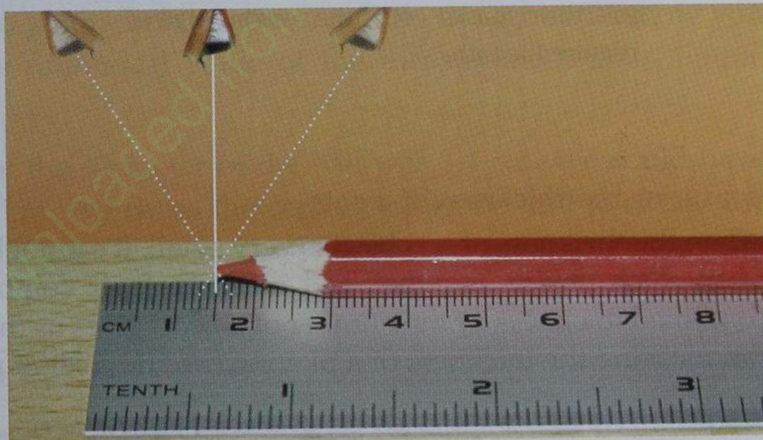
Fig. 2.5 Positioning the eye wrongly causes parallax error.
