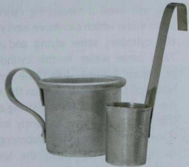
Fig. 2.11 Containers with fixed capacities
