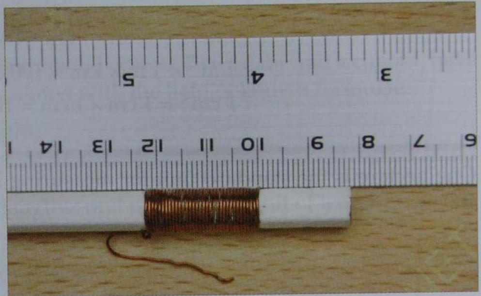
Fig. 2.9 Measuring the diameter of a wire
