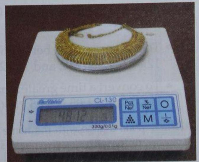
Fig. 2.17 An electronic weighing machine
