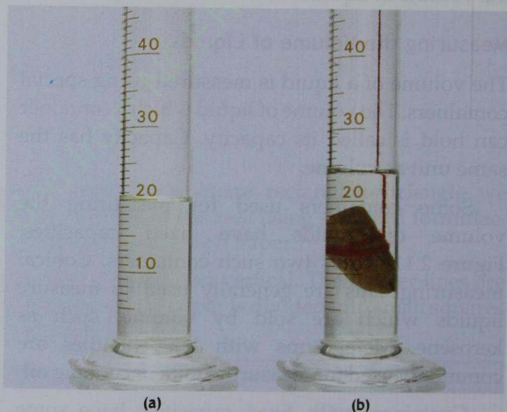
Fig. 2.14 Measuring the volume of a stone
