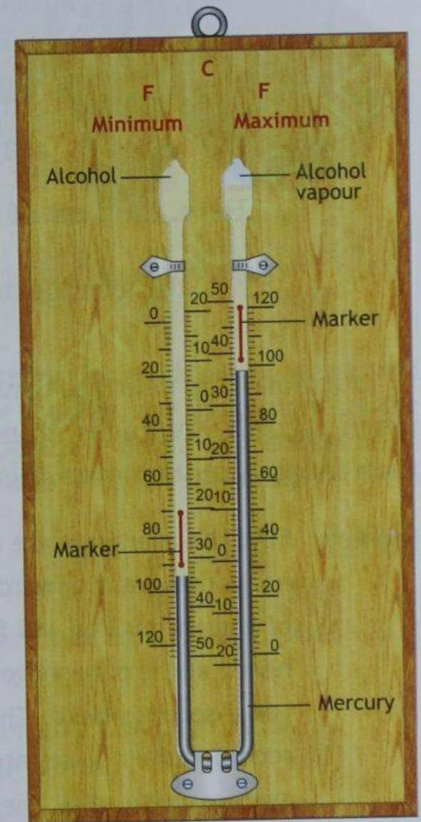
Fig. 2.22 A maximum and minimum thermometer
