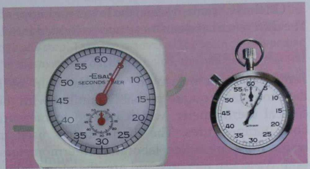
Fig. 2.18 Instruments for measuring intervals of time
