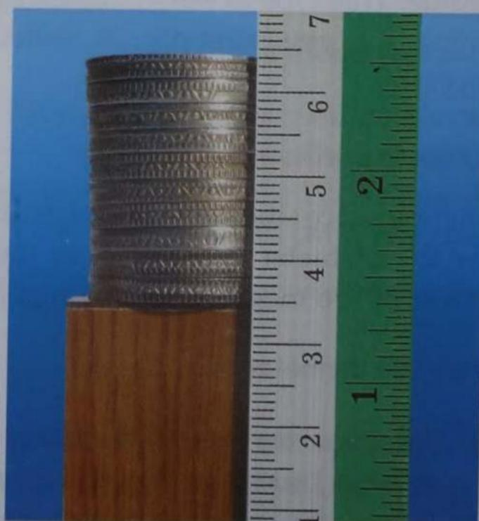
Fig. 2.8 Measuring the thickness of a coin
