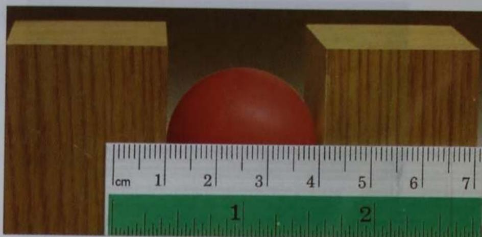
Fig. 2.6 Measuring the diameter of a sphere
