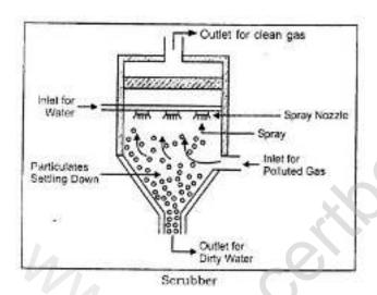
during emissions. In this process, water is introduced into a spray tower by means of a spray nozzle which allow downward flow of water. As the polluted gas flows upwards, the particulates present in the gas collide with the water droplets being sprayed from the spray nozzles. Under the influence of gravitational force, the liquid droplets containing the particulates settle at the bottom.
