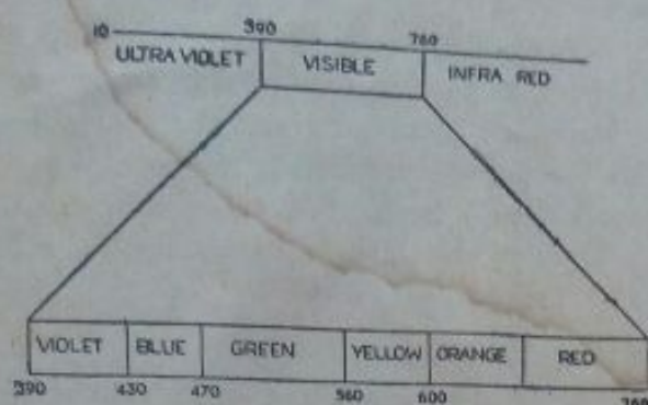
Fig. 29.6 Electromagnetic radiation spectrum.
